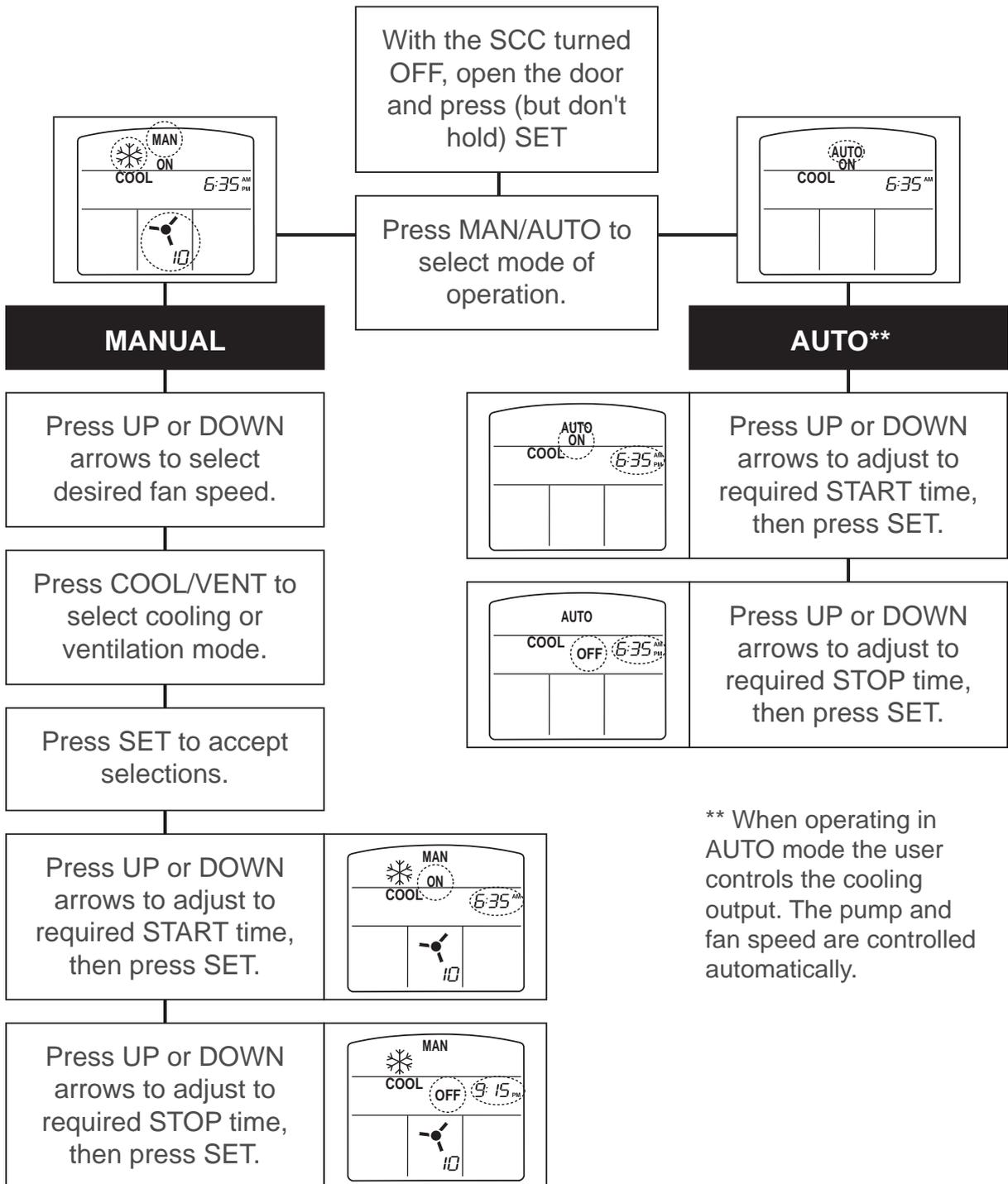
\*\* When operating in AUTO mode the user controls the cooling output. The pump and fan speed are controlled automatically.
