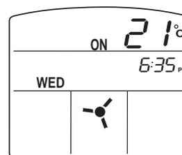
Fan-only display with zones 1, 2 and 3 on - single SCC with zones, or multiple SCC system.
