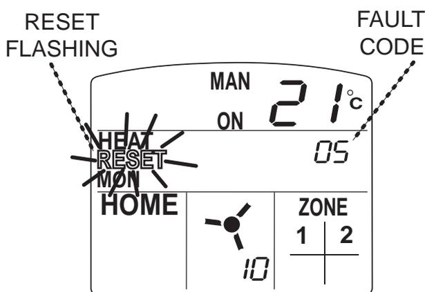
DISPLAY WITH FAULT DETECTED
